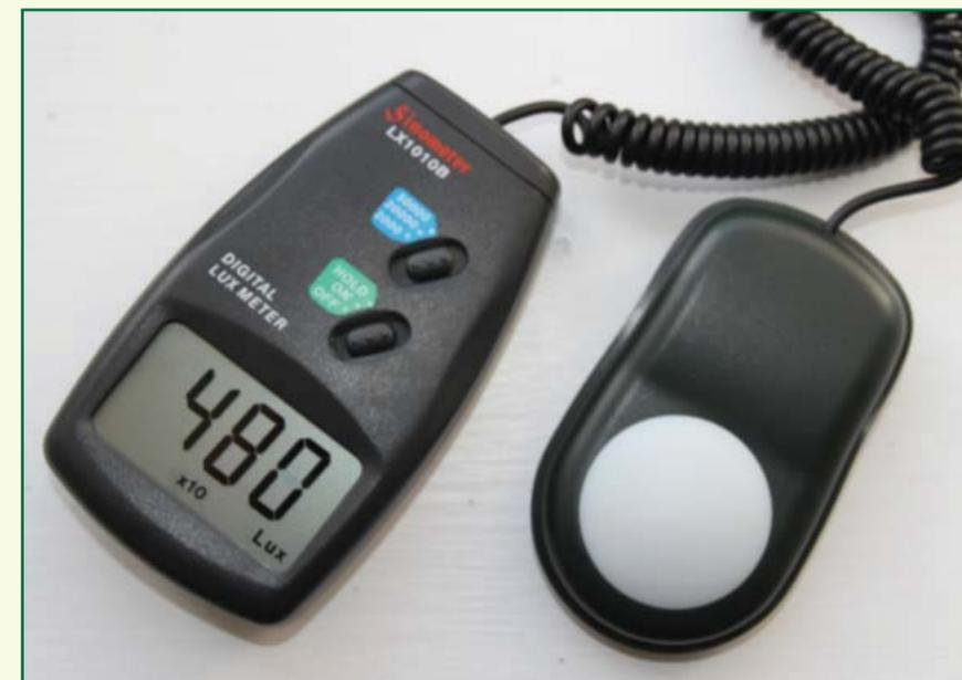
**Neil uses a digital lux meter to check the light in the boxes**
